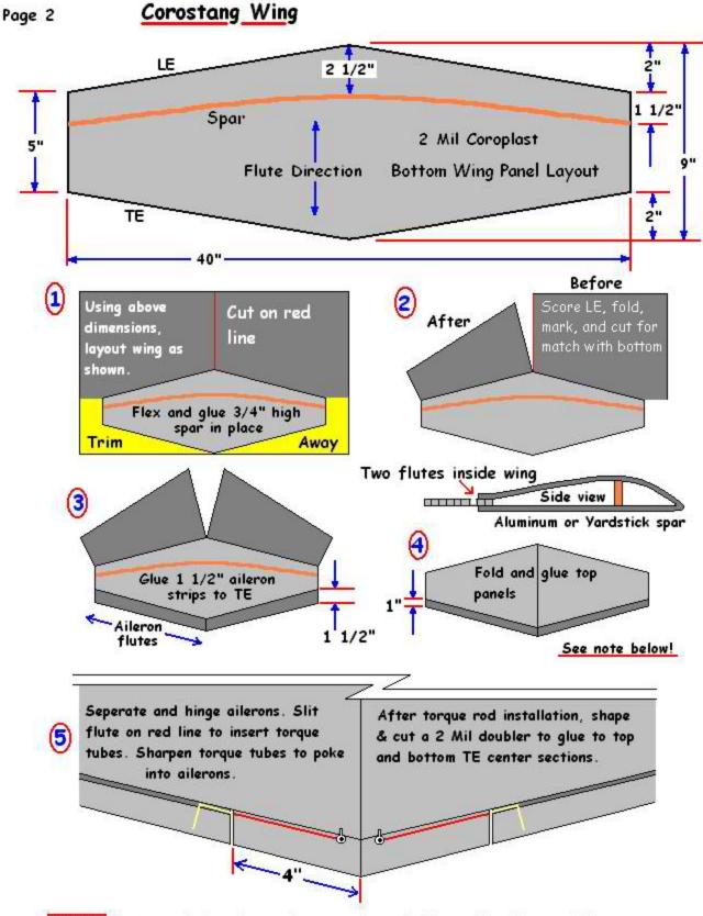
NOTE: Upon completion of step 4, use a piece of thin cardboard or equivilant, cut a notch in it for the spar, insert it into the center section of the wing, and trace your wing's airfoil profile. YOU WILL NEED THIS TEMPLATE FOR FUSELAGE BUILDING!
