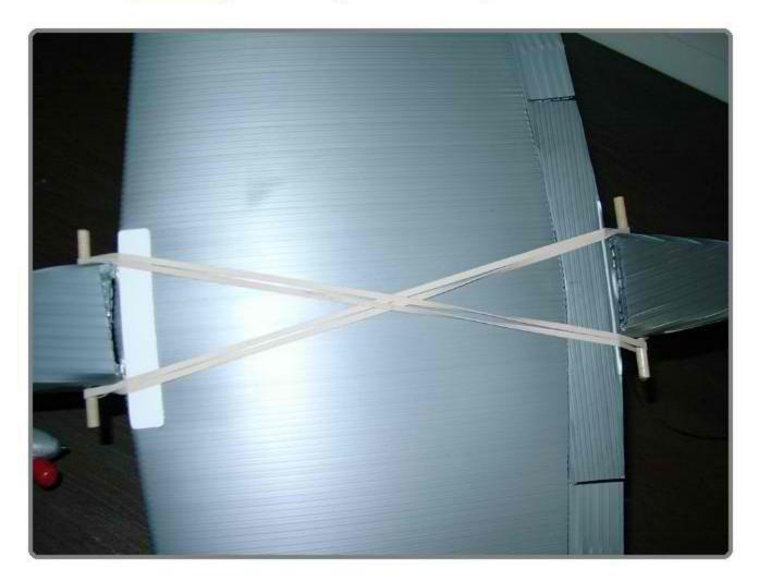
Cut the lower wing center section doubler from 2 mil Coroplast with the flutes running in the chordwise direction, glue in place and insert a piece of coat hanger into a flute as shown. Glue a piece of scrap PVC to the LE area.
